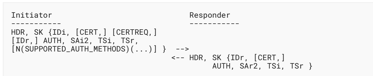
Figure 2: The IKE_AUTH Exchange
